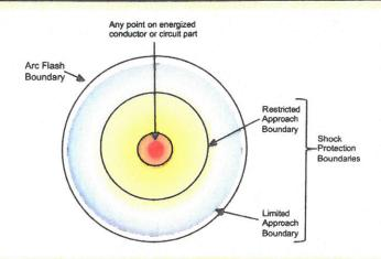
Note: Per NFPA 70E $^{\circ}$  Article 130.5(A) Arc Flash Boundary for systems  $\geq$  50 volts shall be the distance at which the incident energy equals 1.2 cal/cm $^{2}$ .
