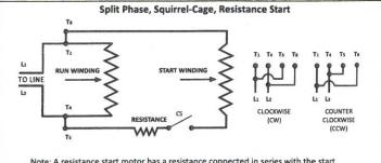
Note: A resistance start motor has a resistance connected in series with the start windings. The centrifugal switch (CS) opens after reaching 75% of normal speed
