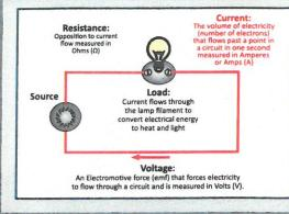
Voltage forces current flow through a resistance. The current returns to the source. There must be a complete path for electrical current to flow.
