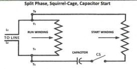
Note: The capacitor start motor is employed where a high starting torque is required. The centrifugal switch (CS) opens after reaching 75% of normal speed.
