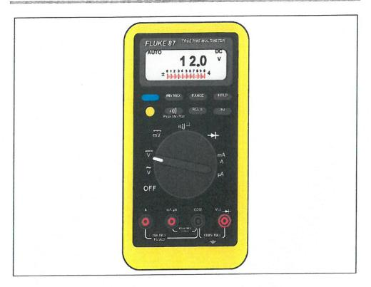
When using the multimeter to make voltage measurements it is important to remember that the voltmeter must always be connected in parallel with the load or circuit under test. The accuracy of the multimeter is approximately  $\pm\,0.01\%$  in the five ac/dc voltage ranges with an input impedance of approximately 10 M $_{\wedge}$  when connected in parallel.
