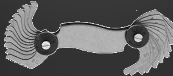
Threads per Inch and Thread Pitch Identifiers
